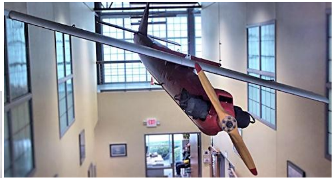
A Radioplane Aerial Target Drone- Used for anti-aircraft gunnery training, pulling a sleeve behind. This drone was used off Camp Haven, and was recovered from Lake Michigan.
